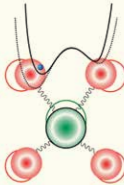
(Left): Snapshot schematic of water molecule, filling oxygen vacancy in the \text{BaCe}_{0.8}\text{Y}_{0.2}\text{O}_{3-\delta} proton conductor. (Right): Lattice vibrations promote proton conductivity.
