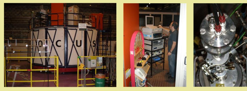
Left: Neutron time-of-flight beamline FOCUS at PSI/SINQ. Middle: Empa researcher setting up a computer macro for electrochemical/neutron in-situ experiments. Right: In-situ cell.
